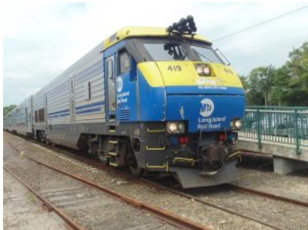
Figure 9. LIRR EMD DE30AC diesel locomotive and consist at Greenport Station (2015: Collection of Derek Stadler)
