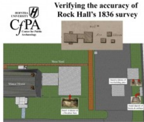
Figure 14: Morris Fosdick's 1836 survey overlaid on Rock Hall Museum's current survey. Note the projected footprint in the west yard of the large kitchen outbuilding that perhaps predates the manor house. The inset photographs show the actual location of the other building features, including the tabby fireplace base as well as features discovered in the far west yard, that align with the 1836 survey. Prepared by Ross T. Rava for the Hofstra University Center for Public Archaeology.
